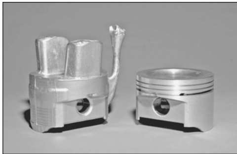
FIGURE 10.16 Aluminum piston for an internal combustion engine: (a) as cast and (b) after machining. The part on the left is as cast, including risers, sprue, and well, as well as a machining allowance; the part on the right is the piston after machining. Source: After S. Paolucci.
