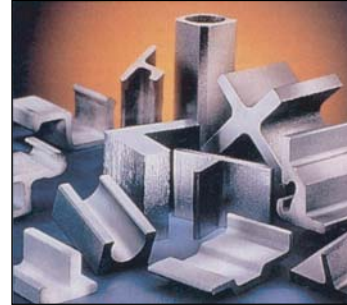
Figure 15.2 Extrusions and examples of products made by sectioning off extrusions.
