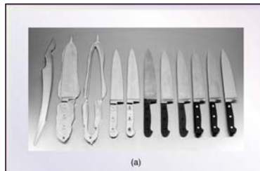
Figure 14.1 (a) Schematic illustration of the steps involved in forging a knife.
